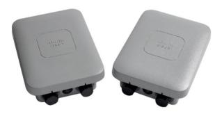
Cisco® Aironet® 1540 Series outdoor access points offer the latest 802.11ac Wave 2 functions in a rugged, ultra-low-profile housing that service providers and enterprises can deploy easily.
